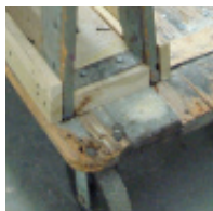
Wood—splinters and rots
